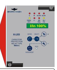
Three-phase overload Earth Fault and unbalance relay with programmable inverse and definite time characteristics suitable for protection, of ungrounded double-wye capacitor banks.
