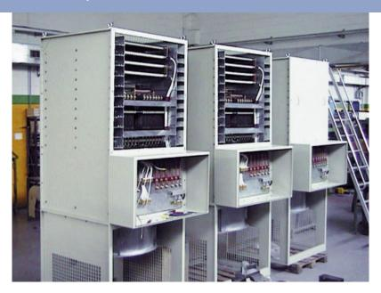
Microelettrica Load Banks can be controlled either locally or remotely (on request), through switches (also manufactured by Microelettrica Scientifica).
