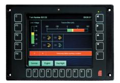
**SIP-32** is a 6.5" DMI with an ARM Cortex-A8 processor and LED backlight. It is a low-cost, mid-performance display, which is preferably used in TCMS applications. The standard interfaces include CAN, Ethernet and USB. Other important features are the long life, the extra robust design of components and housing as well as an attractive design. The SIP-32 is easy to program with PAD.
