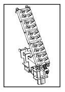
Type B - set of 10 instantaneous contacts (5 N/O + 5 N/C), double interruption molded type, mounted together on a single frame and simultaneously controlled. Each set type B takes the same space as two type P contacts.
