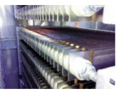
Starting and Braking Resistors are widely employed for controlling motors during start and/or stop.
