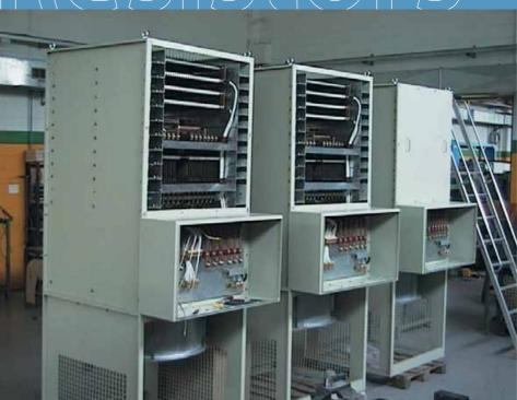
Microelettrica Load Banks can be controlled either locally or remotely (on request), through switches and contactors (also produced by Microelettrica).
