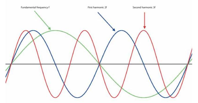
Quality of power is becoming ever more important for both suppliers and end users, as the number of devices that may feed harmonics in power systems is increased, resulting in higher line losses, interferences and resonances. Harmonic Filters - made up by capacitors, inductors and resistors - help clearing harmonics
