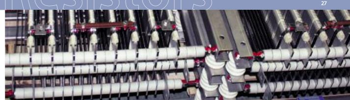
Resistors are designed by our engineers with a 3D model in order to find the best solution for customers and to withstand shocks and vibrations that normally occur in operation without being damaged. Design and all production strictly follow ISO 9001-2008 quality standards and the most severe international specifications.
