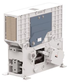
The IR3000V series are single pole, magnetic blow out, trip free, High Speed Circuit Breakers. The closing mechanism is an independent motor operated type. The Circuit Breaker is held closed by an electromagnetic coil or permanent magnet and it is equipped with a direct acting over current trip device which may be either unidirectional or bidirectional. A manual opening device is available as option.
