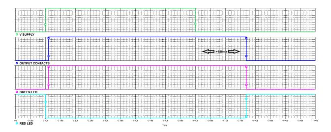
This other graphic shows how an interruption in the supply of less than 150ms has no effect nor in the contact outputs nor in any of the signalisation LEDs:
